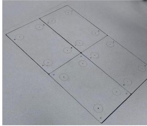
*Figure 5: Force plates to record the weight distribution of patients when undergoing rehabilitation training programmes. Image taken at the Biomedical Engineering department, University of Strathclyde*
