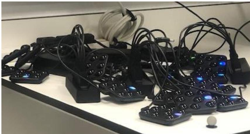
*Figure 4: Clusters with light-up regions identified with a blue colour and wires for the connection to a radiofrequency transmitter. Image taken at the Biomedical Engineering department, University of Strathclyde*
