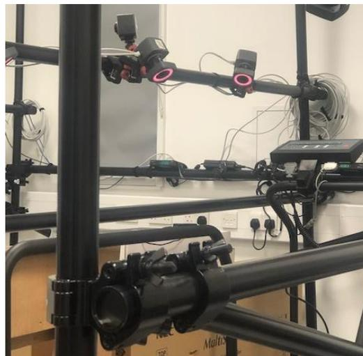
*Figure 1: Attachment of Vicon Nexus visual capture software cameras to treadmill for gait analysis via markers positioned on the body. Image taken at the Biomedical Engineering department, University of Strathclyde*
